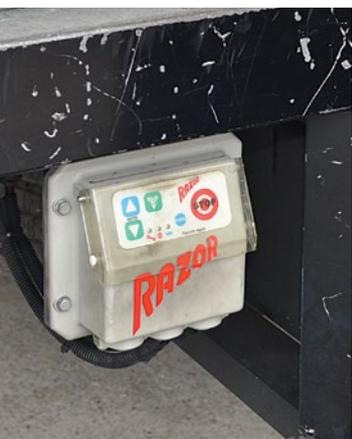
The switch is mounted under the rear, for easy access.
