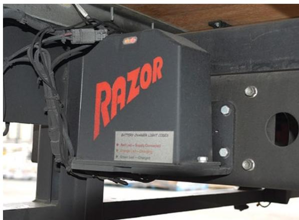
The main battery and charger is mounted out of harm's way under the chassis.
